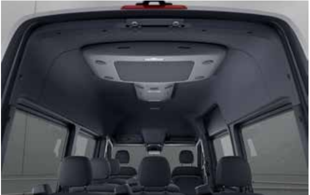
The high-performance overhead air conditioning system supplements the air conditioning in the front with an additional 11 kW of cooling output to deliver the ultimate in climate comfort in the passenger compartment.
