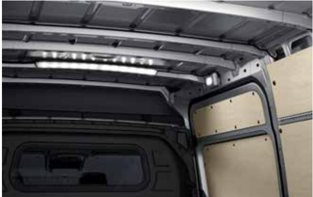
The two LED light strips under the roof illuminate the load compartment, for improved visibility inside when loading and unloading the vehicle.
