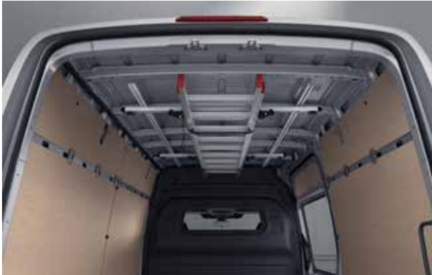
Internally fitted roof racks are available thereby protecting items against theft and preventing the need for external racking to be mounted. 1
