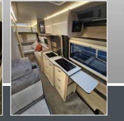
The Altair is an all electric designed motorhome which provides a flexible use anywhere habitation system based on lithium batteries, large solar panels and an inverter which powers all electrical appliances when used in the wild. This motorhome uses no gas. The vehicles drive train is still a diesel engine.
